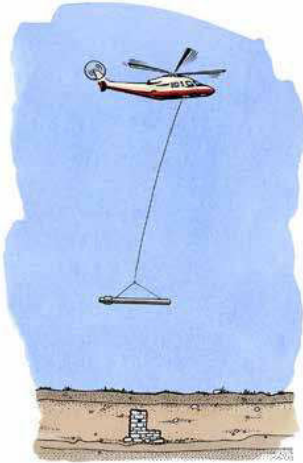
In helicopter geophysics, a so-called "bird" sends electromagnetic waves of different frequencies into the ground. They penetrate the ground at different depths, are reflected and then measured.
